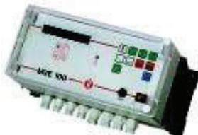
Micro-controlling device **MVE 100** (surface mounting) for the fully automated control of 1-line-demineralisation systems. Fitting for controlling four and five-level-central control valves, pilot distributors or regeneration valves with own regeneration program. Embedded conductivity meter for monitoring the soft water quality and for controlling regeneration sequences.
