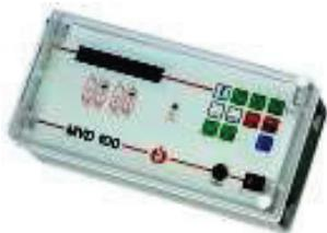
Micro-controlling device **MVD 100** (surface mounting) for the fully automated control of two-line-demineralisation systems. Construction similar to MVE 100, but with inputs for four exchangers and two measuring probes. Current interface 0/4 – 20 mA.
