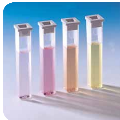
Plastic cells, frosted on two sides, volume 10 ml, path length 13.5 mm, with lid
