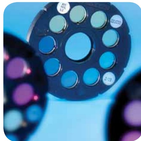
Test disc with colour-stable glass standards
