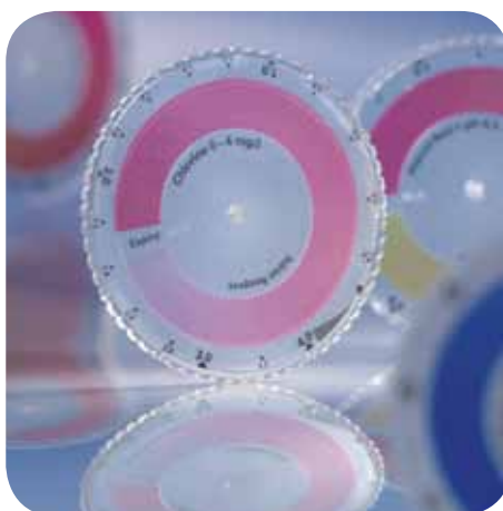
CHECKIT®Discs with continuous colour scales
